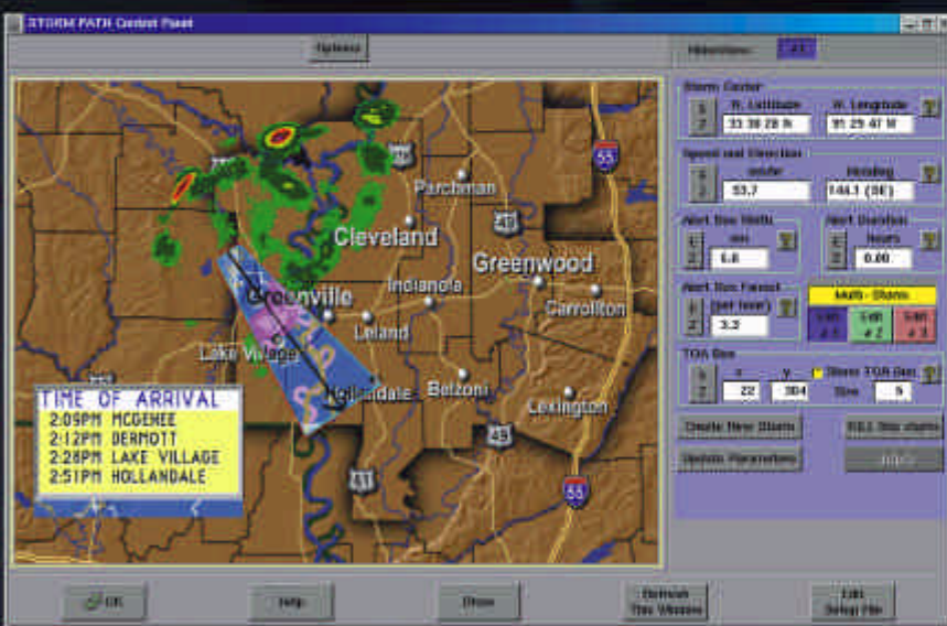
The enhanced Storm Path Analyzer operation allows the creation of new storm paths without stopping the radar sweep.
