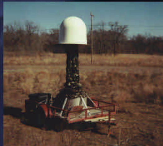
30" System mounted inside a 3.5' radome.
